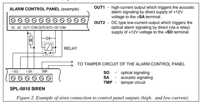
Terminals SA and SO can be connected parallel ("+" to "+" and "-" to "-") for simultaneous work of acoustic and optical signaling.
